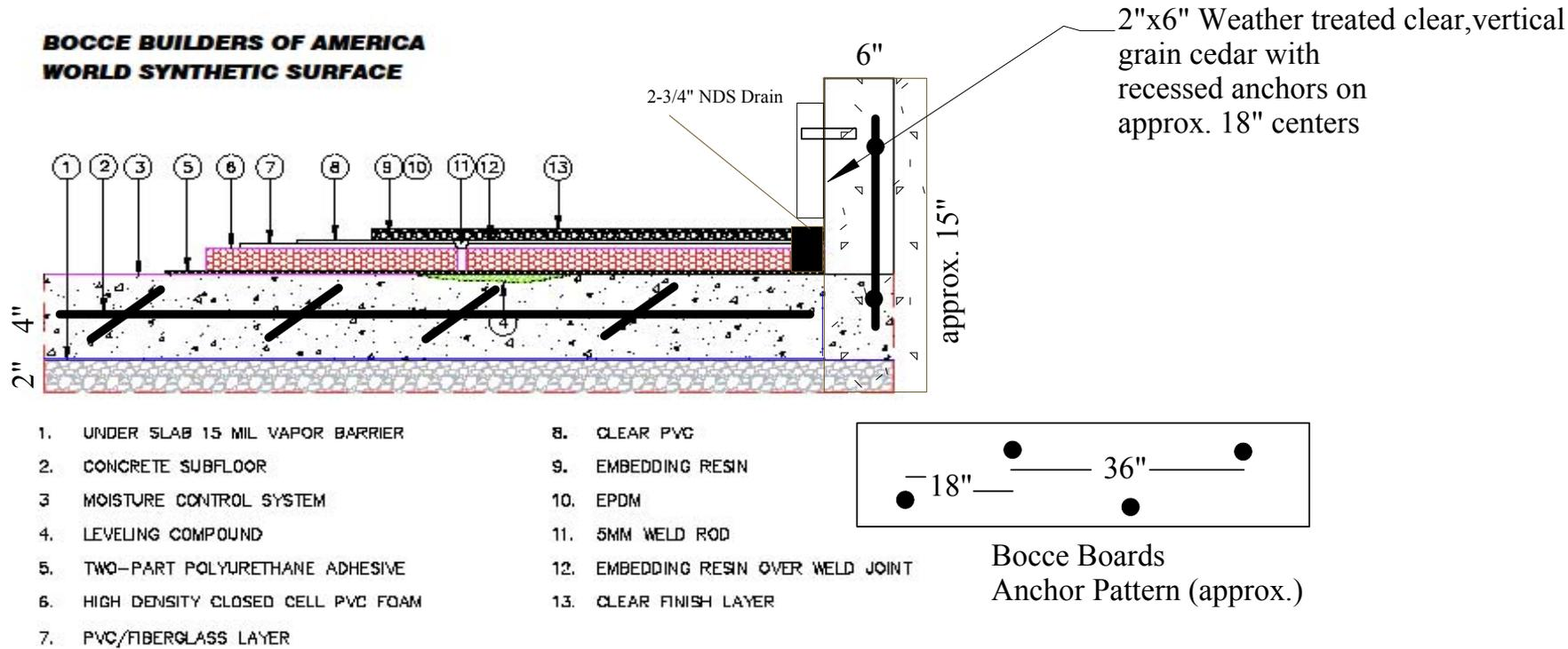
Construction notes: Concrete Stem wall to have 2 horizontal bars of 1/2" steel tied with 3/8" vertical bars on approx. 24" centers
